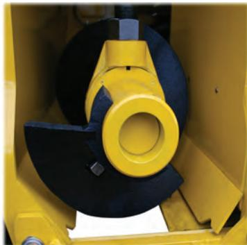
The CP100 is built with conveyor chains that are 25% stronger than pavers in its class, replaceable 3/8" 500 Brinell floor plates, highway class auger bearings and 7/8" 500 Brinell auger flights to give longer lifecycles and better performance. Conveniently located remote greasing points for quick lubrication help keep the paver in optimal shape.
