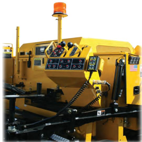
Every CP100 comes with adjustable control consoles that enable operators to find the most comfortable position for operating the paver. Able to tilt down 40° and swing out 30°, operators do not have to trade off comfort for visibility with the CP100.
