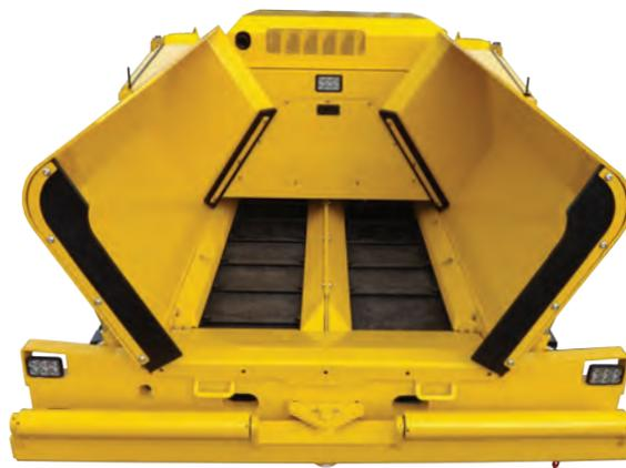
Material is delivered via two horizontally sliding damper doors with adjustable hardened guides for maximum life. This Carlson unique innovation allows a class leading 10" of ground clearance below the augers and keeps obstructions, such as utility boxes, from damaging the damper doors. The adjustability of the opening, combined with class-leading auger flights, contributes to exceptional and even material distribution for better density across the entire width of the screed.
