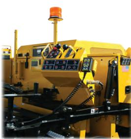
Every CP100 comes with adjustable control consoles that enable operators to find the most comfortable position for operating the paver. Able to tilt down 40° and swing out 30°, operators do not have to trade off comfort for visibility with the CP100.
