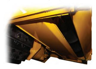
Material is delivered via two horizontally sliding damper doors with adjustable hardened guides for maximum life. This Carlson unique innovation allows a class leading 10" of ground clearance below the augers and keeps obstructions, such as utility boxes, from damaging the damper doors. The adjustability of the opening, combined with class-leading auger flights, contributes to exceptional and even material distribution for better density across the entire width of the screed.
