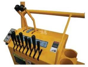
Combined with cup holders, tool trays, boot scrapers and locking tool box all standard, the CP75 leads the way in providing operators a more organized, safer and more comfortable platform. The CP75 also makes end of day clean up easier with its standard 6 gallon (22.7L) wash down system and the elimination of material buildup in the undercarriage with its revolutionary High Flow Material Conveyor.
