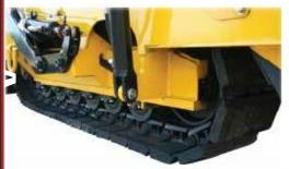
Helping to keep the CP75 running at optimal performance are multiple conveniently located remote greasing stations providing easy daily greasing of vital components. Tension adjustment for the High Flow Conveyor System is also easy with is the High Flow Conveyor tension adjusters located on the exterior of the paver to provide easy access and adjustment.
