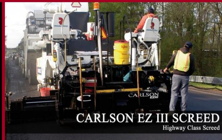
With screed widths available from 8' to 13' 6" and 10' to 17' the front mounted EZ III screed is the choice for highway class paving as well as large commercial applications. The electrically heated screeds are the most technically advanced screeds on the market. With multiple heating elements in direct contact with the screed plate to deliver an even and controllable heat.
