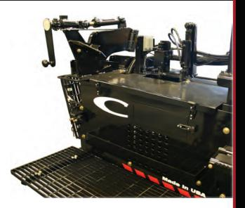
New EZIV's also give operators enhanced versatility with the V3 Endgate platform, a revolutionary design allowing quick changes of runners to suit the requirements of any job. Whether the project calls for joint matching, Safety Edge. or better longitudinal joint density, the V3 endgate's design and heated runners give contractors a proven platform for increasing productivity and decreasing downtime by changing just the shoes rather than entire endgates. perator Focus
