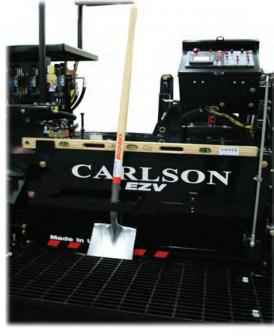
The EZV also gives operators enhanced versatility with the V3 Endgate platform, a revolutionary design allowing quick changes of runners to suit the requirements of any job. Whether the project calls for joint matching, Safety Edge or better longitudinal joint density, the V3 endgate's design and heated runners give contractors a proven platform for increasing productivity and decreasing downtime by changing just the shoes rather than entire endgates.
