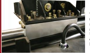
The EZV's extensions are able to maintain their integrity, in part, due to the largest single slide track bushing in the industry for the most surface support. Carlson's single slide track bushings are also adjustable, aiding in maintaining extension rigidity while reducing lifecycle costs. Unlike other screeds in its class, the EZV uses a single hydraulic cylinder per side that is able to slope with the extension, always keeping the cylinder parallel with the chrome rods.
