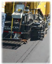
Both the 4" High Density Bolt-on and Sideload Endgate attachments come standard with state-of-the-art heating elements that help increase extrusion of the material while preventing cold spots from forming. And like all of Carlson's screed attachments, the 4" Bolt-on and Sideload Attachment are built with heavy duty components to give operators the instruments to achieve joint density targets season after paving season.
