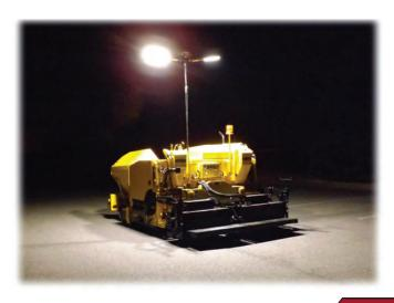
Not only does the LED Blade Light enhance the visibility of and around mobile equipment, it also saves contractors money. Because of the LED's high efficiency and low draw, the platform gains substantial fuel savings over other illumination sources. With increased fuel savings combined with the elimination of replacement costs associated with halogen or high intensity discharge (HID) bulbs, operators are able to see a considerable return on investment with the LED Blade Light.
