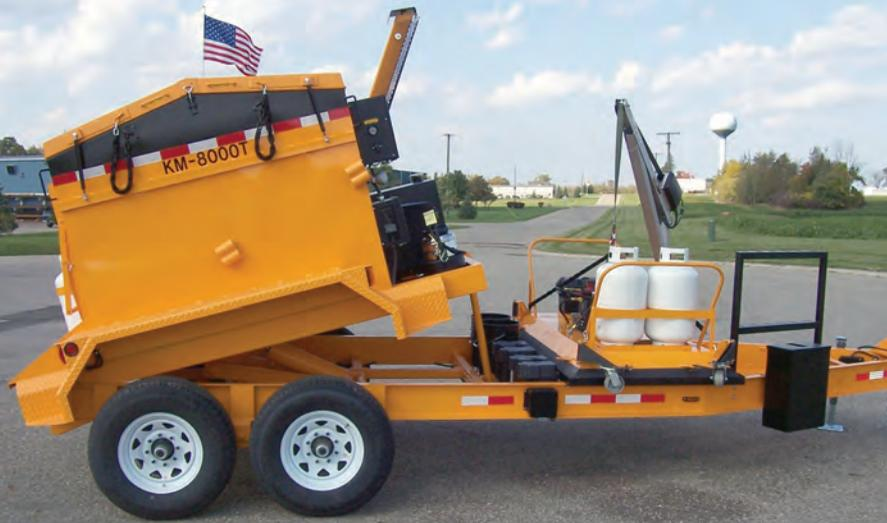
Diesel unit shown with on-board KM 2-18X infrared, hydraulic dump and other options.
